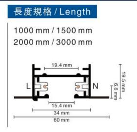
2-circuit main voltage track in extruded aluminum. Main voltage 220-240V. Electrical wiring is located in an extruded PVC insulated housing. The track is supplied with a series of accessories which will successfully resolve almost all types of lighting installation requirements. And also has the facility for direct surface mounting through knockouts at 500m spacing.
