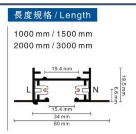
2-circuit main voltage track in extruded aluminum. Main voltage 220-240V. Electrical wiring is located in an extruded PVC insulated housing. The track is supplied with a series of accessories which will successfully resolve almost all types of lighting installation requirements. And also has the facility for direct surface mounting through knockouts at 500m spacing.
