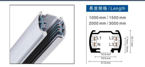
4-circuit main voltage track in extruded aluminum. Main voltage 220-240V. Electrical wiring is located in an extruded PVC insulated housing. The track is supplied with a series of accessories which will successfully resolve almost all types of lighting installation requirements. And also has the facility for direct surface mounting through knockouts at 500m spacing.
