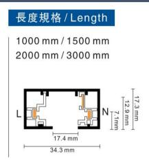
3-circuit main voltage track in extruded aluminum. Main voltage 220-240V. Electrical wiring is located in an extruded PVC insulated housing. The track is supplied with a series of accessories which will successfully resolve almost all types of lighting installation requirements. And also has the facility for direct surface mounting through knockouts at 500m spacing.
