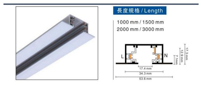
3-circuit main voltage track in extruded aluminum. Main voltage 220-240V. Electrical wiring is located in an extruded PVC insulated housing. The track is supplied with a series of accessories which will successfully resolve almost all types of lighting installation requirements. And also has the facility for direct surface mounting through knockouts at 500m spacing.
