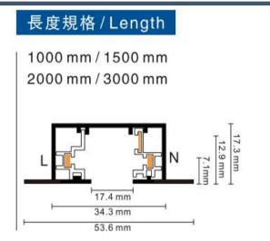
3-circuit main voltage track in extruded aluminum. Main voltage 220-240V. Electrical wiring is located in an extruded PVC insulated housing. The track is supplied with a series of accessories which will successfully resolve almost all types of lighting installation requirements. And also has the facility for direct surface mounting through knockouts at 500m spacing.
