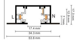
3-circuit main voltage track in extruded aluminum. Main voltage 220-240V. Electrical wiring is located in an extruded PVC insulated housing. The track is supplied with a series of accessories which will successfully resolve almost all types of lighting installation requirements. And also has the facility for direct surface mounting through knockouts at 500m spacing.
