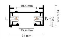
4-circuit main voltage track in extruded aluminum. Main voltage 220-240V. Electrical wiring is located in an extruded PVC insulated housing. The track is supplied with a series of accessories which will successfully resolve almost all types of lighting installation requirements. And also has the facility for direct surface mounting through knockouts at 500m spacing.
