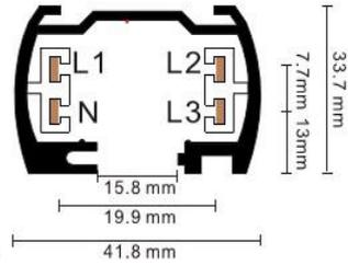
4-circuit main voltage track in extruded aluminum. Main voltage 220-240V. Electrical wiring is located in an extruded PVC insulated housing. The track is supplied with a series of accessories which will successfully resolve almost all types of lighting installation requirements. And also has the facility for direct surface mounting through knockouts at 500mm spacing.
