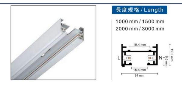
2-circuit main voltage track in extruded aluminum. Main voltage 220-240V. Electrical wiring is located in an extruded PVC insulated housing. The track is supplied with a series of accessories which will successfully resolve almost all types of lighting installation requirements. And also has the facility for direct surface mounting through knockouts at 500m spacing.
