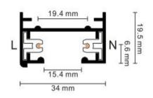
2-circuit main voltage track in extruded aluminum. Main voltage 220-240V. Electrical wiring is located in an extruded PVC insulated housing. The track is supplied with a series of accessories which will successfully resolve almost all types of lighting installation requirements. And also has the facility for direct surface mounting through knockouts at 500m spacing.
