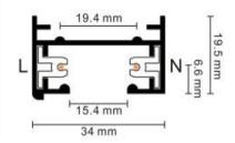
2-circuit main voltage track in extruded aluminum. Main voltage 220-240V. Electrical wiring is located in an extruded PVC insulated housing. The track is supplied with a series of accessories which will successfully resolve almost all types of lighting installation requirements. And also has the facility for direct surface mounting through knockouts at 500m spacing.
