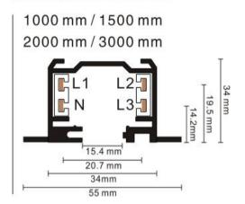
4-circuit main voltage track in extruded aluminum. Main voltage 220-240V. Electrical wiring is located in an extruded PVC insulated housing. The track is supplied with a series of accessories which will successfully resolve almost all types of lighting installation requirements. And also has the facility for direct surface mounting through knockouts at 500m spacing.
