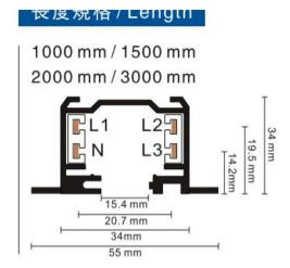
4-circuit main voltage track in extruded aluminum. Main voltage 220-240V. Electrical wiring is located in an extruded PVC insulated housing. The track is supplied with a series of accessories which will successfully resolve almost all types of lighting installation requirements. And also has the facility for direct surface mounting through knockouts at 500m spacing.
