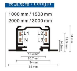
4-circuit main voltage track in extruded aluminum. Main voltage 220-240V. Electrical wiring is located in an extruded PVC insulated housing. The track is supplied with a series of accessories which will successfully resolve almost all types of lighting installation requirements. And also has the facility for direct surface mounting through knockouts at 500m spacing.
