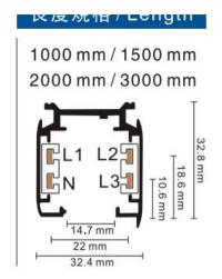
4-circuit main voltage track in extruded aluminum. Main voltage 220-240V. Electrical wiring is located in an extruded PVC insulated housing. The track is supplied with a series of accessories which will successfully resolve almost all types of lighting installation requirements. And also has the facility for direct surface mounting through knockouts at 500m spacing.
