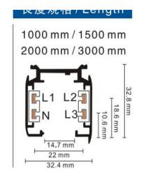
4-circuit main voltage track in extruded aluminum. Main voltage 220-240V. Electrical wiring is located in an extruded PVC insulated housing. The track is supplied with a series of accessories which will successfully resolve almost all types of lighting installation requirements. And also has the facility for direct surface mounting through knockouts at 500m spacing.
