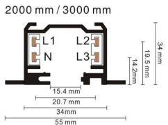
4-circuit main voltage track in extruded aluminum. Main voltage 220-240V. Electrical wiring is located in an extruded PVC insulated housing. The track is supplied with a series of accessories which will successfully resolve almost all types of lighting installation requirements. And also has the facility for direct surface mounting through knockouts at 500m spacing.
