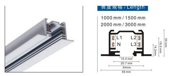
4-circuit main voltage track in extruded aluminum. Main voltage 220-240V. Electrical wiring is located in an extruded PVC insulated housing. The track is supplied with a series of accessories which will successfully resolve almost all types of lighting installation requirements. And also has the facility for direct surface mounting through knockouts at 500m spacing.
