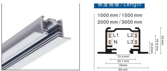
4-circuit main voltage track in extruded aluminum. Main voltage 220-240V. Electrical wiring is located in an extruded PVC insulated housing. The track is supplied with a series of accessories which will successfully resolve almost all types of lighting installation requirements. And also has the facility for direct surface mounting through knockouts at 500m spacing.
