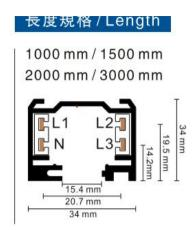
4-circuit main voltage track in extruded aluminum. Main voltage 220-240V. Electrical wiring is located in an extruded PVC insulated housing. The track is supplied with a series of accessories which will successfully resolve almost all types of lighting installation requirements. And also has the facility for direct surface mounting through knockouts at 500m spacing.
