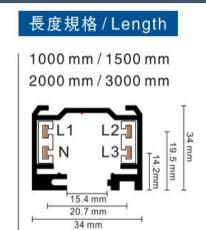
4-circuit main voltage track in extruded aluminum. Main voltage 220-240V. Electrical wiring is located in an extruded PVC insulated housing. The track is supplied with a series of accessories which will successfully resolve almost all types of lighting installation requirements. And also has the facility for direct surface mounting through knockouts at 500m spacing.
