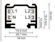
4-circuit main voltage track in extruded aluminum. Main voltage 220-240V. Electrical wiring is located in an extruded PVC insulated housing. The track is supplied with a series of accessories which will successfully resolve almost all types of lighting installation requirements. And also has the facility for direct surface mounting through knockouts at 500m spacing.
